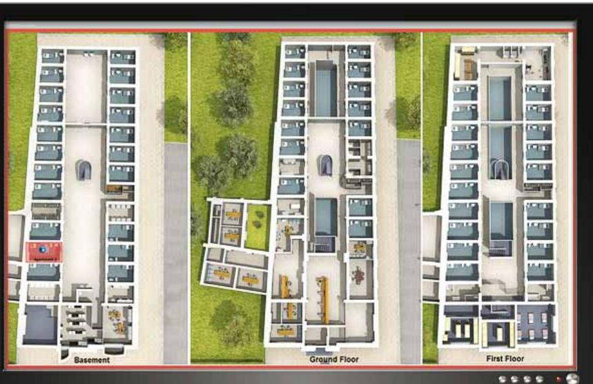
**Graphical Display** – Custom graphics can be prepared using our YAAM software. The graphics provide staff with a clear image where assistance is required within the building at a glance of an eye. YAAM software is able to use a range of sounds and colours to distinguish the various levels of alert to help staff access the priority of active events.
